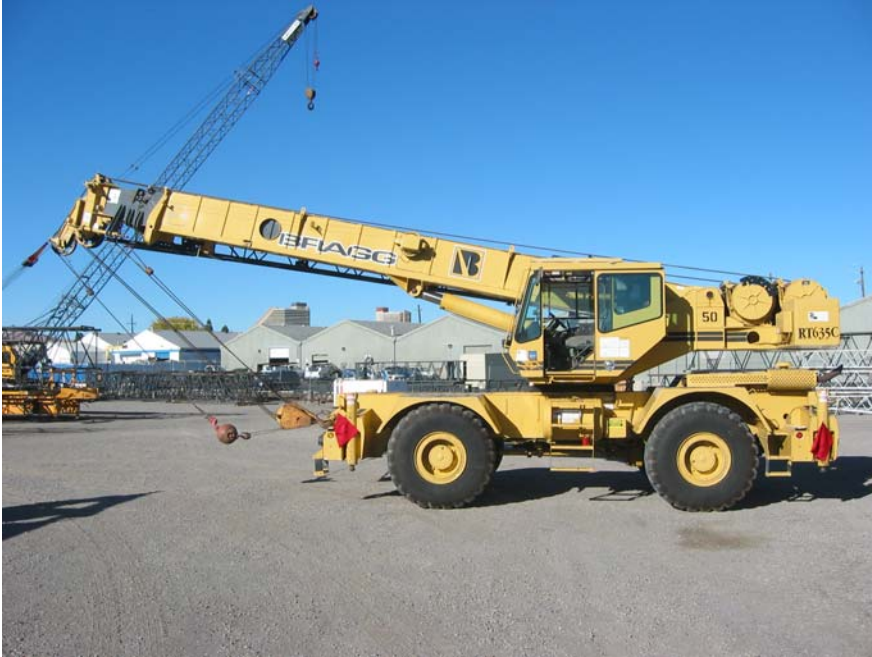
1993 Grove RT600C (RT635C) 35-ton Rough Terrain Crane 105' main boom with 29' of jib and weighs 65,000 pounds
