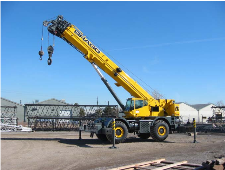
(2) 2004, (1) 2007 Grove RT890E 90-ton Rough Terrain Crane 141' main boom with 56' of jib and weighs 93,400 pounds + 22,000 pound counterweight
