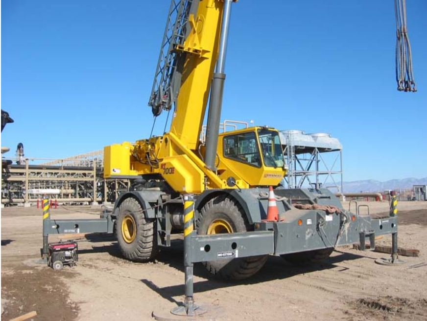
2006 Grove RT700E (RT760E) 60-ton Rough Terrain Crane 110' main boom with 56' of jib and weighs 90,000 pounds
