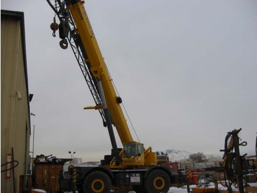
2004 Grove RT875 75-ton Rough Terrain Crane 128' main boom with 56' of jib and weighs 90,300 pounds + 18,000 pound counterweight
