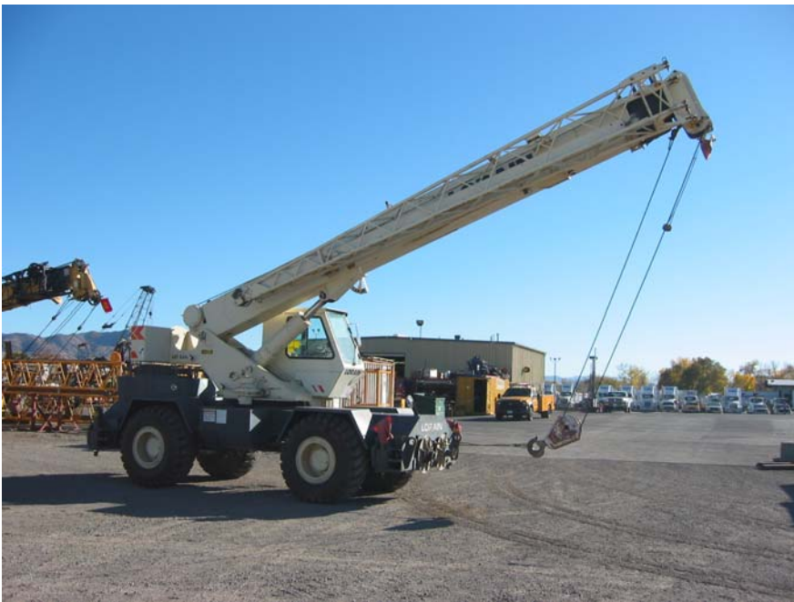
1994 Lorain LRT-230E 30- ton Rough Terrain Crane 94' main boom with 43' of jib and weighs 56,500 pounds
