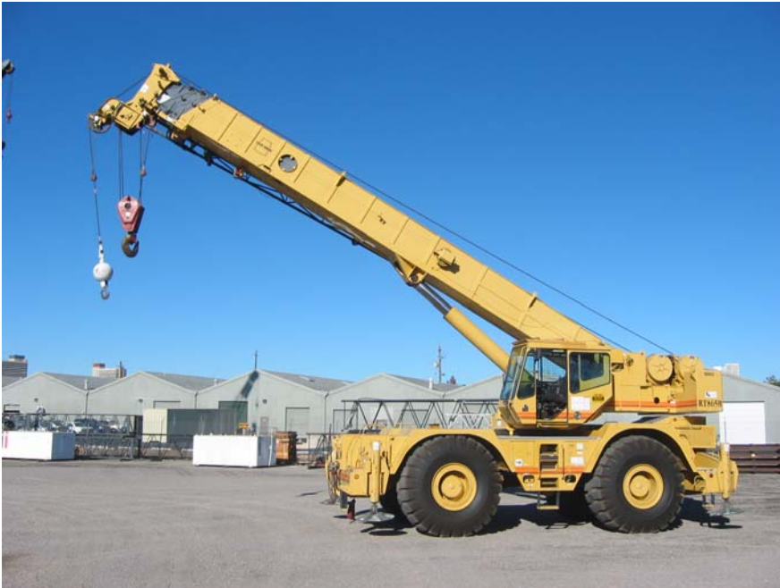
1995 Grove RT865B 65-ton Rough Terrain Crane 125' main boom with 35' of jib and weighs 107,000 pounds
