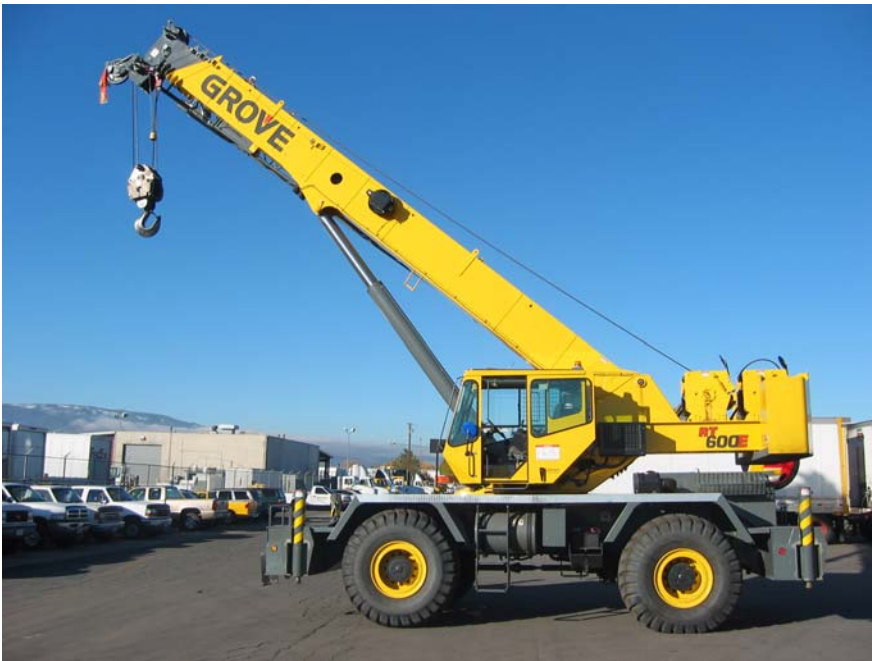
2006 and 2007 Grove RT600E (RT650E) 50-ton Rough Terrain Crane(s) 105' main boom with 51' of jib and weighs 77,000 pounds
