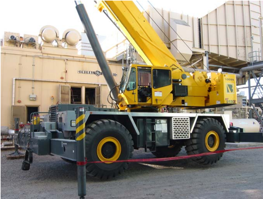
2008 Grove RT9130E 130-ton Rough Terrain Crane 160' main boom with 59' of jib and weighs 129,000 pounds + 40,000 pound counterweight
