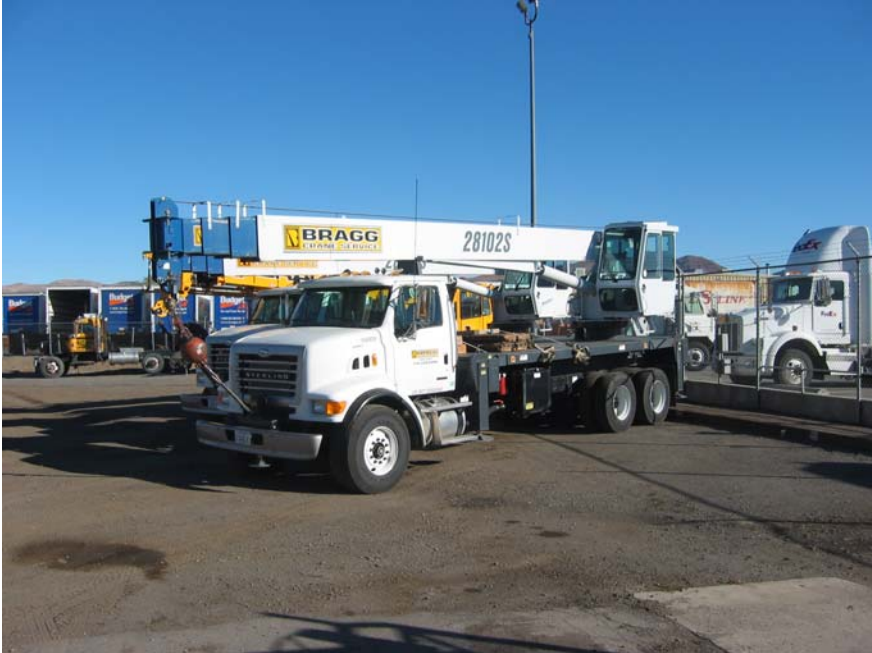
(2) 2006 Manitex 28102S 28-ton Boom Truck 102' main boom with 46' of jib
